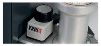
Head's Assembly Adjustment. Nexus comes as standard with an additional knob to set the height of the tool to prevent denting (kiss-cut) the material.
