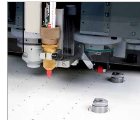
Three independent heads. Manual regulation of the cut depth in increments of just 0,1 mm (1/32") allows better control during cutting when working with materials of different thicknesses. The maximum thickness permissible is 5mm (3/16"). (3)
