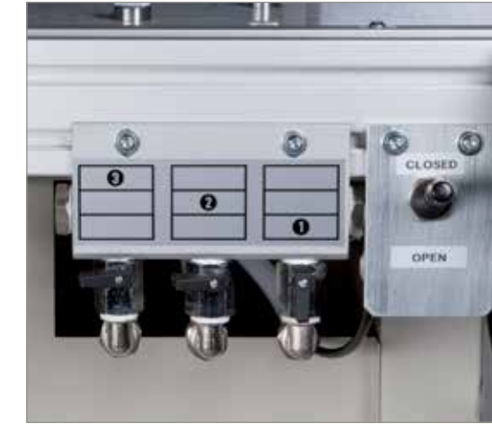
Vacuum table with independent workstations. The Geminus is fitted with 6 macro areas subdivided across the two workstations.
