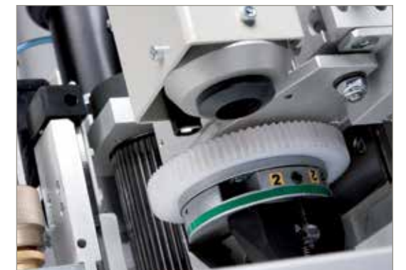
Digital camera for crop mark detection.
