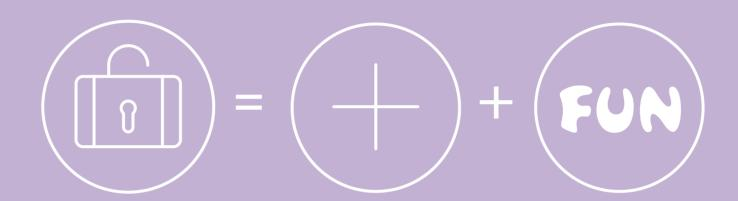
Press Mand + for half a second to remove travel lock. Press Mand - for half a second to activate it again.
