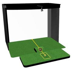
Minus 15 inches from this measurement. For example: if you measure 130 inches tee to screen, input "115" into the "Tee to Screen Distance" dialog.
