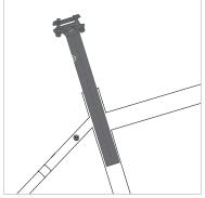
Figure 1 - Correct Installation
