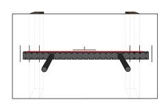
Align the center of the bracket to the center line you marked on the wall. Align the bracket to the horizontal line.
