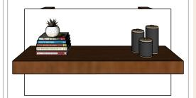
Slide shelf onto bracket and check the fitting. Your shelf should fit tight and may require additional force.
