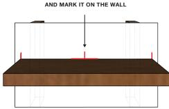
With a measuring tape, find the center of the shelf and mark the center on the wall. There may be a marking
