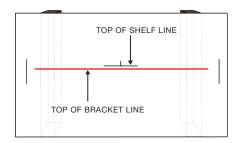
With the bracket in the shelf, measure the distance from the top of the shelf and the top of the bracket. Using a level, draw a horizontal line where the top of the bracket would be placed.
