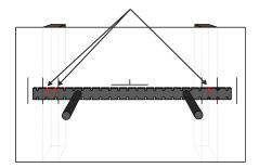
Install the bracket using wood screws to the marked studs on the wall. Drill screws along the top of the bracket. Bottom screws are optional.
