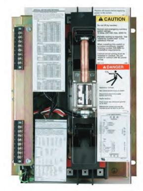
■ Switch mechanism, including contact assemblies, is UL 1008 certified to verify suitability for applications requiring high endurance switching capability for the life of the transfer switch. Withstand and closing ratings are validated using the same set of contacts, further demonstrating the robust nature of the design.
