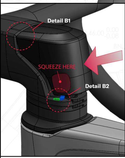
B. Place Stem Cover by aligning cable hole pegs at front of cover (B1) with Cable passage holes in stem. Squeezing Cover at grip indication surface (B2), continue to push forward until tabs snap into place in topsteerer spacer.
