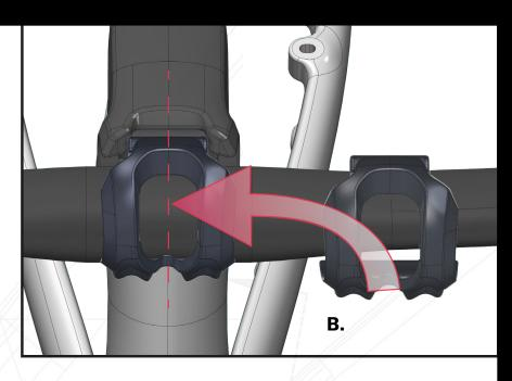
**B.** Start with faceplate over tapered portion of bar top moving it inwards and laterally until centered on bar
