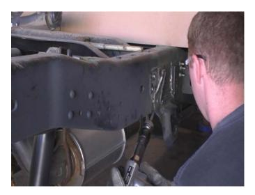
11. Grind the frame smooth and install the spring hanger in the existing rivet holes.
