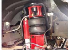
7. Install the air bag assembly just as the coil spring came out. Use the original lower mounting bolt and supplied spacer to attach the lower mount to the axle housing.
