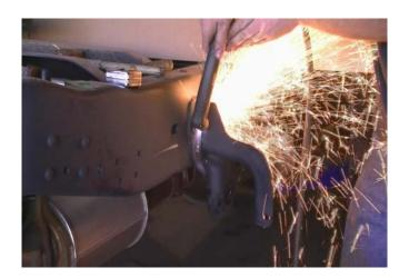
9. After the outside of the hanger is removed, use a grinder with a cut off wheel to cut the welds attaching the hanger to the frame. Be sure to only cut the weld and do not cut into the frame.
