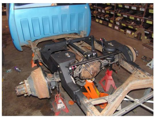
Street Scraper completely installed with truck still on jack stands
