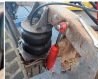
Install Lower bag mounts on top of axle. 4Link bars will attach to lower bag mounts. Relocate factory shocks, or buy replacements from us #1321 Loop/Loop for rear.
