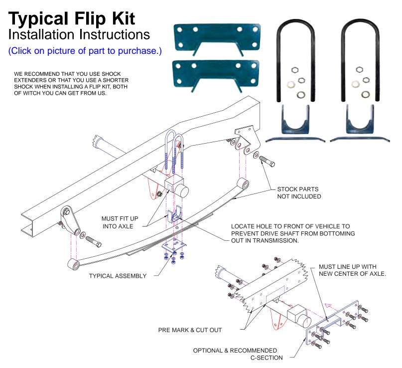
NOTE: KIT WILL LOWER A STOCK TRUCK 5-6". THE TRUCK BED MUST BE REMOVED TO INSTALL. STOCK LEAF SPRINGS WILL BE RELOCATED BELOW THE REAR AXLE. AN OPTIONAL C-SECTION MUST BE PURCHASED TO NOTCH AND REINFORCE THE FRAME RAILS ON GM 88 & UP AND ON FORD F-150 TRUCKS.
