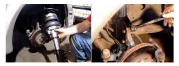
On many of our struts, you might find an extra set of mounting holes on the bottom Clevis. For the lowest position, select the top holes.
