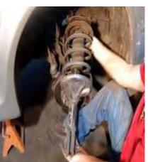
Remove Factory Strut. In most cases, you will reinstall the top bearing plates shown below.
