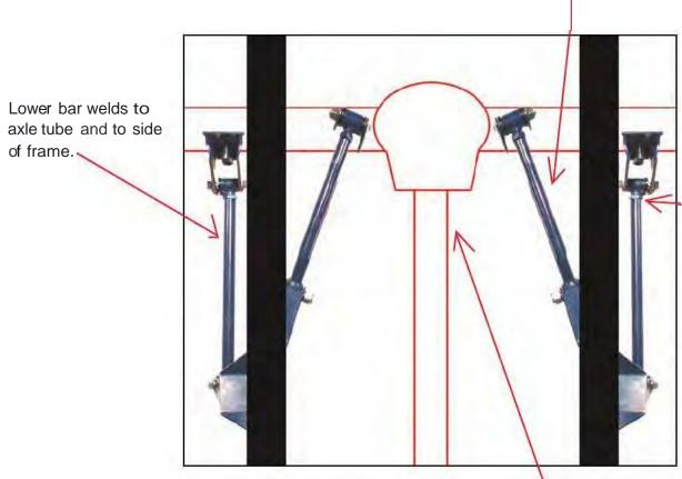
We recommend having adjustment bushings set in middle location before welding mount to axle or frame.
