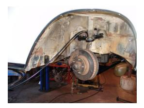
6. Install the upper and lower control arms, cycle the suspension to make sure there is no binding and that the suspension moves freely.
