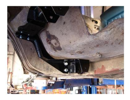
8. Install the main upper cross member in the car. It will fit tight against the floor pan and will also attach to the brackets that were installed in the previous step. Note that the driveshaft tunnel will need to be modified to allow adequate clearance when the suspension is fully deflated.
