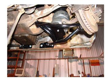
5. Install the airbag and upper bag mount assembly in the spring pocket. Note that the fitting and air line need to be attached to the bag before the bag mount is installed
