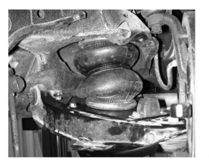
Bolt the lower air spring plate to the lower arm. The two outer holes will align with the factory bump stop holes. The inner two holes must be drilled.
