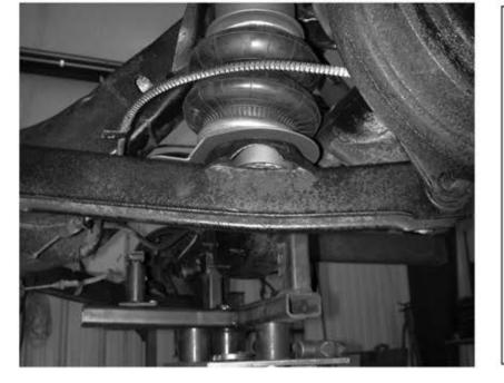
10. Bolt the lower mount to the bottom of the air spring using a 3/8" x 3/4" bolt, lock washer and flat washer. Before tightening, make sure it aligns with the lower arm.
