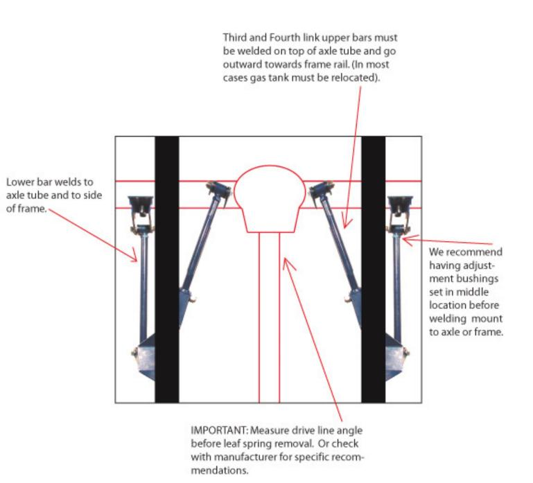
Caution: We recommend tack welding link bars in place and moving vehicle up and down to ensure nothing binds before permanently welding 4 link in place.
