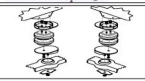
Typical Rear for cars/trucks with Coilsprings Remove or trim/modify bumpstops as necessary Brackets we sometimes send extra top brackets so y
