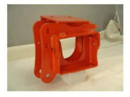
11. The inside of the frame needs a little bit of trimming before the upper bag mounts can be put on. Use a cut off wheel or a plasma cutter to cut a straight line. Trim the inside lip of the frame so the bag mount will fit flush against the bottom of the frame
