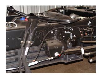
7. Install the new 4 link mounts. The 4 link mounts install into the factory leaf spring
