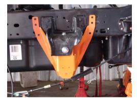
8. Install a 9/16"-12 x 4 ½" bolt with the included machined steel reducers in the factory leaf spring mounting hole. Make sure the 4 link mount is straight and square on the frame. Tighten the bolt to secure the position of the hanger and mark and
