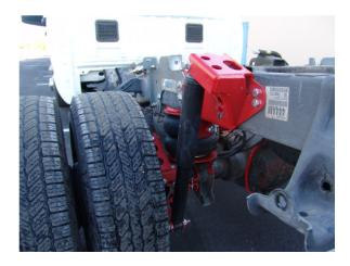
19. The factory brake line may need slight modification in order to allow enough clearance for the lower shock mount. Carefully use a grinder to modify the caliper so the brake line can be turned 90 degrees
