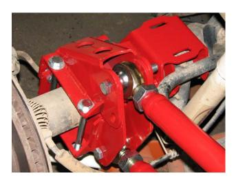
11. Attach the lower bag mount to the axle and install the 4 link bars
