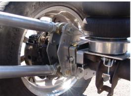
16. Install air fitting on airbag and mount the rear air bags. Be sure to place the 9 ½" diameter flat bag plate between the bag and bag mounts. This keeps the bag from rolling over itself at low pressures and contacting any sharp objects.
