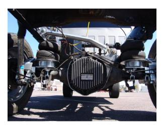
14. Install the pan hard bar with the bushing end on the frame and the heim joint at the axle
