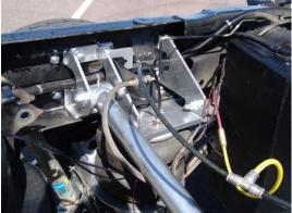
10. The rear shock mounts have provisions to install directly over 2 existing rivets that attach the rear cross member to the frame. Mark and drill the holes and attach the rear shock mounts.
