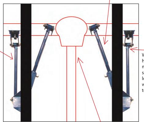
We recommend having adjustment bushings set in middle location before welding mount to axle or frame.
