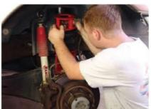
With the brackets bolted to the air bag, the assembly was slipped into place just as the coil spring had been. The factory bolt is used in conjunction with a supplied spacer to attach the lower mount to the axle.
