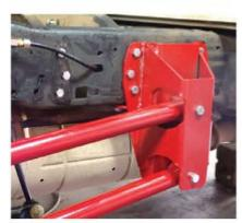
In the rear, the leaf springs were supported, and then unbolted. The front spring hanger was removed, and the fourlink mount was bolted in. The mount utilizes the front holes of the old leaf spring hanger, and the rear holes were marked and drilled. The links were adjusted to the correct length and installed. The pinion angle is adjustable via the rod ends.
