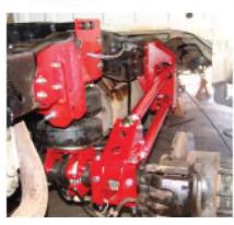
6 Spacers are provided to fit on the recessed area of the frame before the panhard bar bracket is installed. The panhard bar mount uses four existing holes in the frame. Just as with the front link mount, additional holes needed to be marked and drilled.
