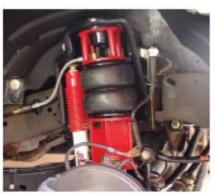
Here, the front suspension is completely installedit took less than 10 minutes. Note the included steel leader hoses-those are ideal protection from possible wheel rub or wear.
