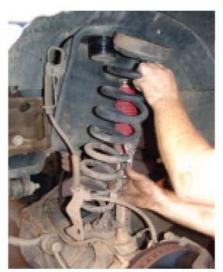
First, the lower bolts of the front-end shocks were removed. That allowed the axle to extend far enough for the coil spring to be removed, along with the lower spring perch and rubber isolator.
