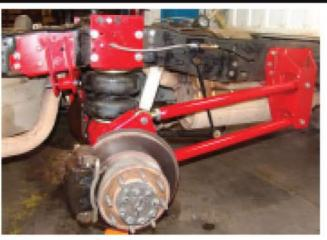
Here is the complete rear suspension. The factory shocks, sway bar, and exhaust are retained. Pretty efficient!
