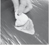
Lift or hold the section of torn foam. Use the paint brush and Mat Glue to apply the adhesive to all of the exposed foam area. Allow the glue to dry for approximately 10 minutes.
