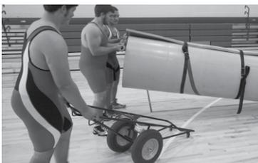
Resilite sells a mat EZ-Lifter Bar to assist when lifting a rolled mat section. The EZ-Lifter Bar allows two (2) people to safely lift one end of a standard mat section, allowing a mat cart to be placed under the mat.
