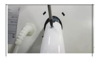
After taking off the cover you're going to have to remove the top screw with a philips head screw driver. You might need to use a hammer to apply pressure on the arm to take it out. They are not meant to come out once they are installed so you will need to use some force.
