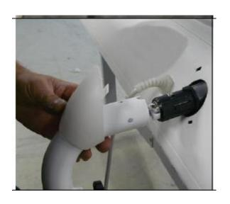
First remove the circular white plastic cover by using pressure to pop it out as shown in the picture.
