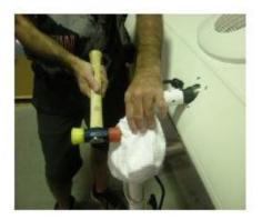
Take the new part provided to you and replace the plastic cover onto the pole. Then place it into the canopy body where you previously removed it. You might need the hammer to push it back in, as shown. Use a rag so it does not scratch.
