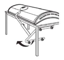
Place the arm into the base as shown. You will need to use a lot of force in order to get the shock to jump into position. If you do not use enough force the unit will not higher and lower, and you will not be able to attached the screws in the next step.
