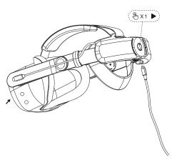
Power button is designed for activating the smart charging on the Quest 3. To charge the strap individually, leave the power button in the" Off" position after plugging it into charge.
