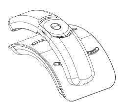
Charging: LED flashes at current power level Fully Charged: LED1-4 lights up
