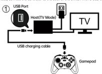
2.After the wired connection is successful, unplug the USB cable, and press the "Home" button then the controller will automatically connect wirelessly.
