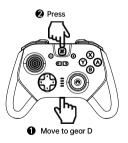
5.Mode switch: Double-click the pairing button to switch to D-input mode. When set successfully, the controller vibrates for 1s, and LED1+LED2 is on.
