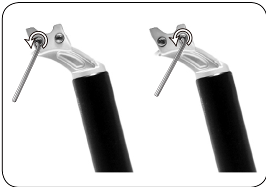
Step 1 - With a 4mm Allen wrench, loosen the Kore I-beam seat rail clamp
