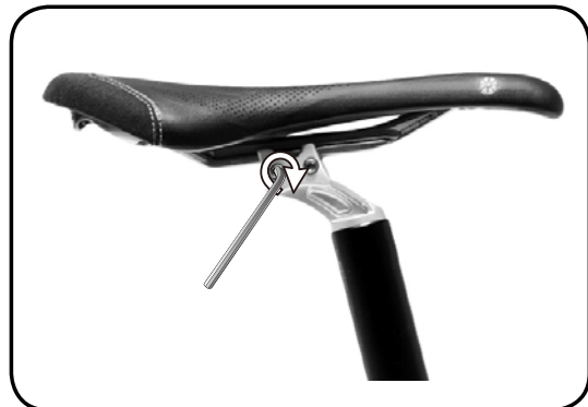
Step 5 - Tighten the pre-greased bolts to 85 in/lbs or 9.5 NM.
