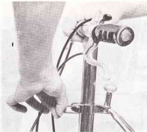
12. Release handlebar quick release clamp and adjust the height; clamp handlebar in proper position. (Warning: Always be certain handlebar post and brace are properly and securely fastened.)
