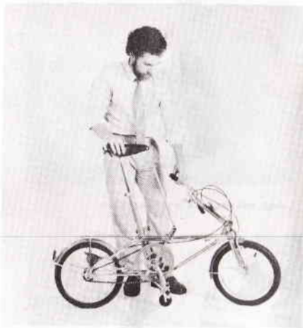
9. Raise handlebar to vertical position, while twisting it slightly to the right.
