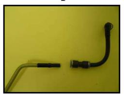
Use original nylon hose with connector and attach with supplied union to the Lines To Go nylon hose.
