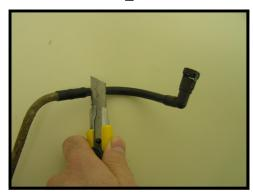
Cut original nylon hose in the same position as Lines To Go nylon hose.
