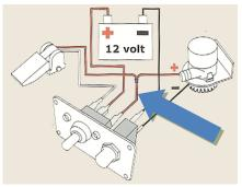
A typical bilge system. Connect the blue wire to the positive side of the bilge pump.
