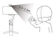
(Note: The best distance of gesture control is between 0.5 and 1.5 meters (1.6 - 5 ft). Make sure that both gesture and face are shown in front of Al sensor within this range.)
