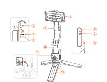
1 Power Button (Mode Switching) 2 Battery Indicator Light ③ Working Mode Indicator Light ④ Bluetooth Indicator Light (5) Phone Clamp (Built-in 360° Infinite Rotary Motor) 6 Reset (Force Shutdown) Type C Charging Port 8 Motor Lock 9 Rotary Joint 10 Extendable Stick 11 Remote Control
