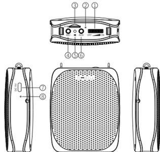
**1.Power switch & volume control:** Rotate the knob to "ON" to turn on the amplifier, the operation indicator will light up. Rotate to "ON" continuously to increase the volume, rotate to "OFF" continuously to decrease the volume till turn off.
