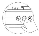
1.Switch on the amplifier and press "M" to enter into Bluetooth mode. The Bluetooth mode is ready with voice prompt "Bluetooth is waiting for connection".
