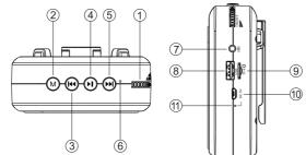
1.Power switch & volume control: Rotate the knob to "ON" to turn on the amplifier when the power indicator is blue. Rotate to "ON" continuously to increase the volume, rotate to "OFF" continuously to decrease the volume till turn off.
