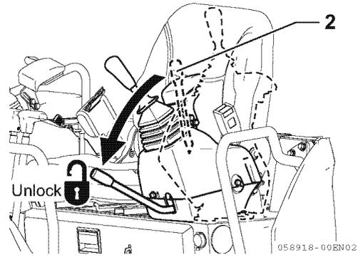
4. Set the lock lever **2** to the "LOCK" position to lock the control levers and pedals.
