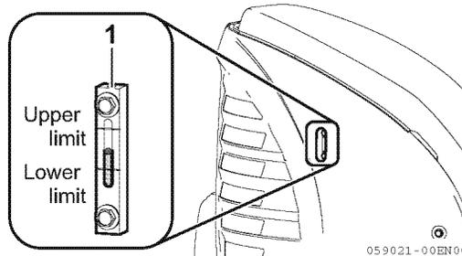
3. Open the bonnet B 2 and lock it with the stopper 5. Replenish oil from the oil supply port 3 if the oil level is below the lower limit.
