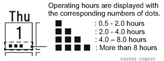
Pressing the F2 switch ◀ or F3 switch ▶ will change a selected date to another, allowing checking of the operational status of the machine in the past 90 days.
