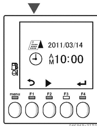
Pressing the F2 switch ► will highlight the year displayed on the screen. Press the F3 switch ⊕ repeatedly to increase the value by one until the desired value is reached.
