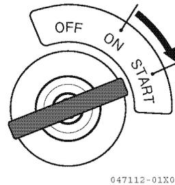
4. After the engine has started, release the starter switch key. The starter switch key will return to the "ON" position by itself.
