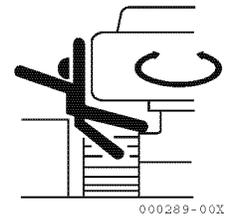
**Take measures to prevent the machine from getting stuck before working on soft ground**
