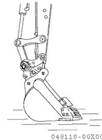
3. Set up the handle of the lock pin.
