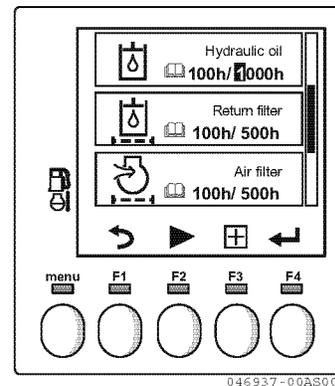
3. After highlighting the digit to be changed, press the F3 switch
