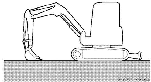
2. Lower the attachment onto the ground.
