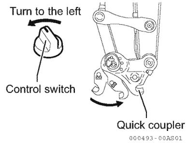
8. Remove the quick coupler from the attachment.
