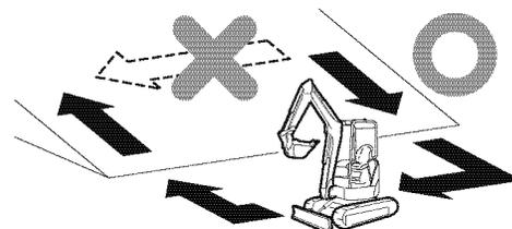
**Level the ground of the work site and the area within which the machine travels**
