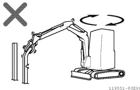
■ **Do not run the machine with an object held by the attachment mounted on the implement**
