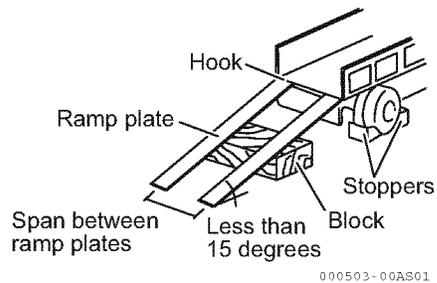
The ramp plates should be set at an angle of less than 15 degrees.
