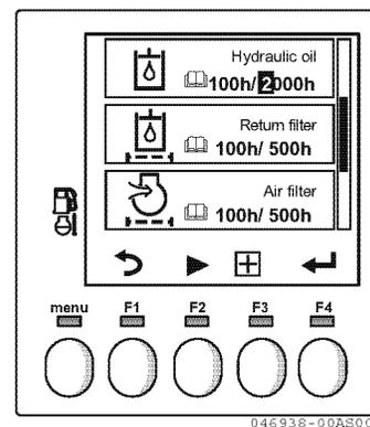
4. After completion of the change of maintenance intervals by repeating Steps 2 and 3, pressing the F4 switch
