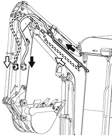
\* During single acting operation, the side shown by the black arrow is under high pressure.
