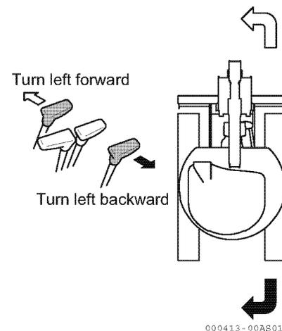
■ **Steering the machine while traveling
