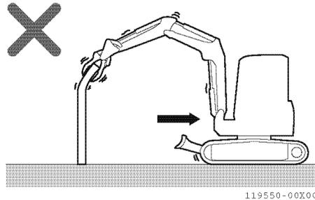
■ **Do not turn the upperstructure with an object held by the attachment mounted on the implement**
