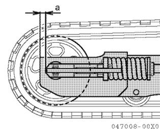
7. If the tension is loose even after grease injection, it is necessary to replace the rubber track or the grease adjuster. Contact your dealer and ask for replacement.
