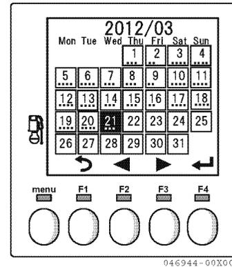
The machine operating hours for each day are displayed roughly with the corresponding numbers of dots under the date number.
