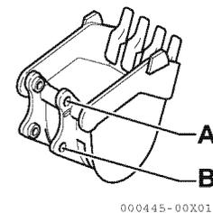
5. Clean the bucket boss section and install the O-ring.
