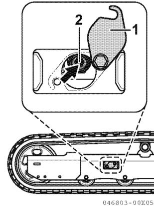
2. Raise the machine using the implement and inject grease through the greasing valve 2 using a grease gun until the rubber track tension is within the specified value of 0.3 to 0.5 in. (8 to 13 mm).
