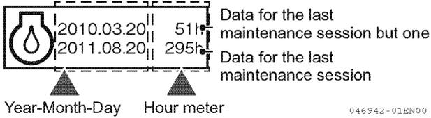
Maintenance items are displayed in vertical alignment on the LCD screen.
