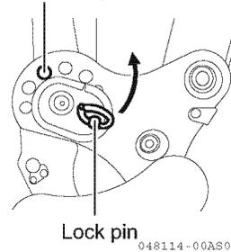
8. Turn the arrow on the lock pin to the lock side.
