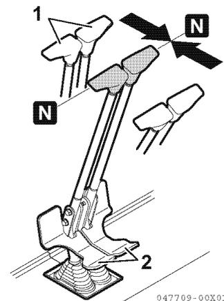
2. Move the engine speed control lever 3 or turn the engine speed control dial 3 to the IDLING position.
