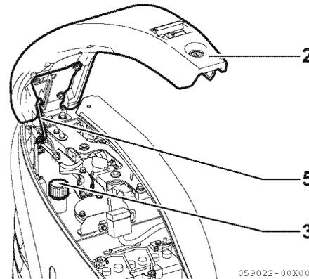
4. Disengage the stopper 3 and close the bonnet B 2.
