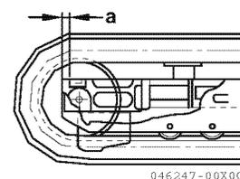
6. The tension can be adjusted until the clearance "a" is reduced to 0 in. (0 mm). If the tension is still loose after adjustment, the pin and the bush should be reversed or replaced because they are worn excessively. Ask your dealer to repair the track.
