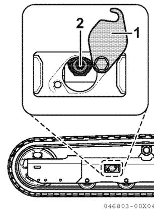
4. Insert the steel pipes into the rubber track and turn the sprocket in the reverse direction. When the rubber track is separated from the idler by the steel pipes, slide the rubber track off.
