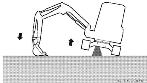
4. Check the rubber track tension again. If the tension is improper, adjust it again.
