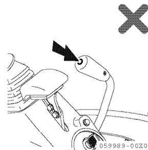
2. Move the engine speed control lever or turn the engine speed control dial to IDLING position.
