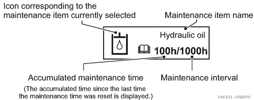
Maintenance items are displayed in vertical alignment on the LCD screen.
