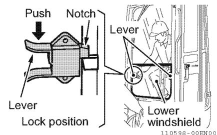
1. Push the right and left lock levers to the arrowed direction and slowly lift the lower windshield up to the upper lock position.
