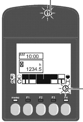
**Information icon** | This icon is displayed to indicate the existence of information. Pressing the F4 switch allows checking of information details.
