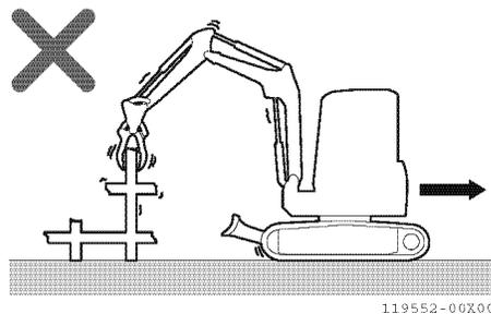
■ **Do not lift a load using the attachment mounted on the implement**
