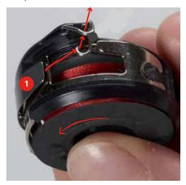
> Hold the bobbin case so that the thread guide points upward.
