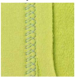
The visible hem is especially suitable for elastic hems in jersey, cotton, wool, synthetic and mixed fibers.
