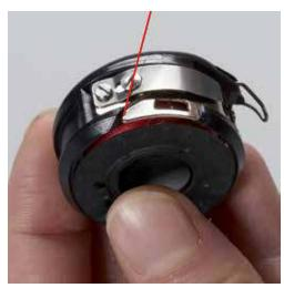
> Pull the thread to the right under the spring (1), then lead the thread under the thread guide and pull upwards.
