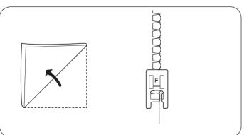
Use a lightweight fabric (tricot, for example). Fold the fabric as shown and stitch on the fold. Allow the needle to just pierce next to the folded edge to create a Vari-Overlock edge. The thread tension may need to be increased slightly.
