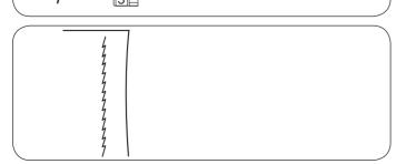
This stitch is a narrow stretch stitch designed to eliminate puckering on knit fabrics and bias seams, while permitting the seam to be pressed completely open flat.
