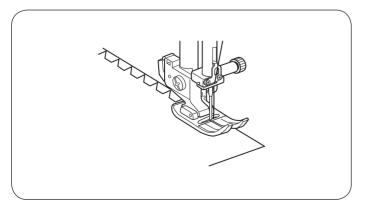
Carefully guide the fabric so the needle falls off the edge when it swings to the right.
