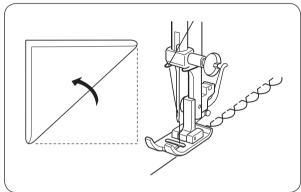
Use a lightweight fabric such as tricot. Fold the fabric and stitch on the bias. You may need to increase the needle thread tension slightly. Allow the needle to just clear the folded edge of the fabric at zigzag stitches.
