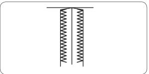
Simple zigzag stitching is used to finish raw edges (overcasting) on most fabrics in order to prevent fraying. This is the fastest way to finish an edge.
