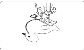
Baste (or fuse with iron-on fabric joiner) appliqué pieces on the fabric.
