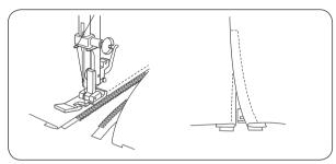
Pin or baste zipper tape to fabric and place it under the foot.
