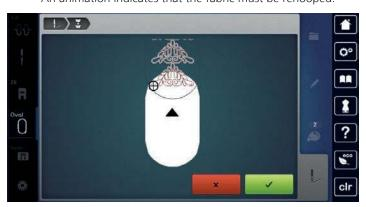
> Remove the hoop and rehoop the fabric so that the stitched out reference points are in the upper part of the area to be embroidered and at least 3 cm from the top edge of the hoop.
