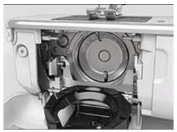
> Give one drop of oil in each of the two oil depots so that the felts are damp and make sure that the redmarked surface of the hook sleeve remains free of oil.
