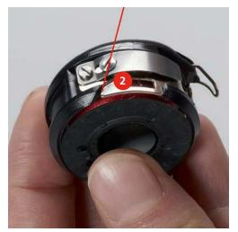
> Pull the thread to the right under the spring (3), then lead the thread under the two thread guides (4) and pull upwards.
