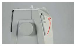
Inserting foam pad and thread spool The foam pad prevents the thread from getting hooked at the swiveling spool pin.
