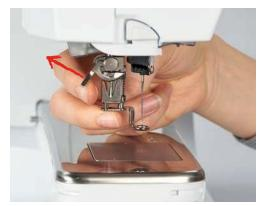
> Press the clamping lever down.
