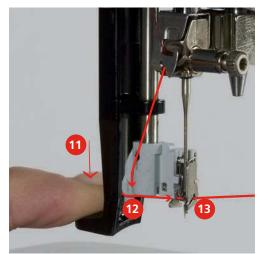
> Release the lever and the thread simultaneously to thread.
