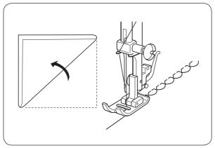
Use a lightweight fabric such as tricot. Fold the fabric and stitch on the bias. You may need to increase the needle thread tension slightly. Allow the needle to just clear the folded edge of the fabric at zigzag stitches.
