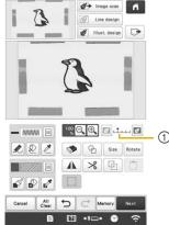
\* After the scanned image is converted to stitching, it appears as a background in the pattern drawing screen. Use gauge ① to adjust the transparency of the background. Each touch of Illustration pattern darker. Each touch of Idarkens the background, making the illustration pattern lighter.
