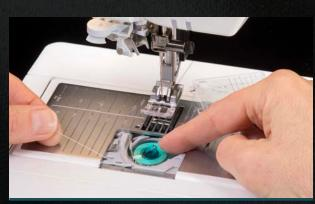
With the extra-large bobbin you can stitch your projects with less interruptions. You can also wind a bobbin while still sewing using the separate bobbin winding motor. No need to stop and unthread your needle.
