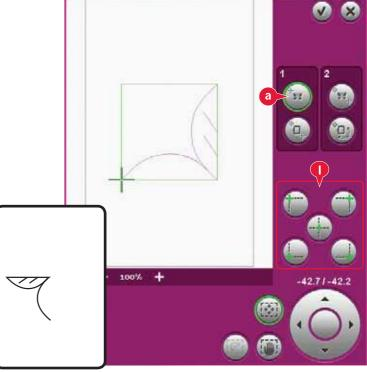
1b. Select the next function, place locking point on fabric (b), to move the locking point on the screen to the right position in the hoop.
