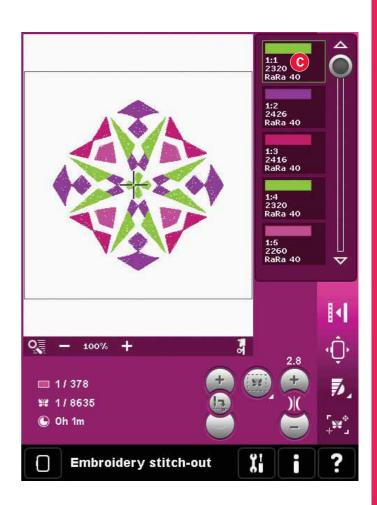
7. Clear sufficient space to accommodate movement of the embroidery arm and the hoop. Hold the needle thread and touch the start/stop button (D) or the foot control. The machine starts embroidering.
