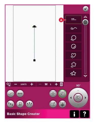
3. Select touch function - scale, and adjust the line to desired length by touching and dragging on screen or using the arrows in the wheel.
