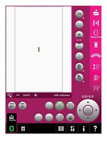
2. Open Basic Shape Creator™ feature. Select the straight line from the list (A). Select touch function - rotate, and then touch the wheel center one time to rotate the baseline 90 degrees.
