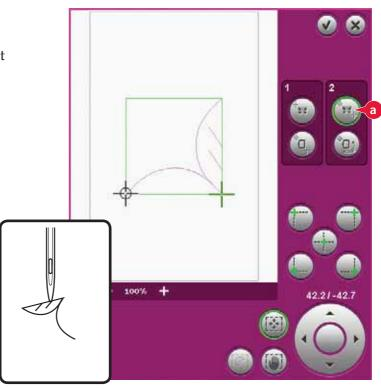
2b. Select the next function, select maching point on fabric (b) to move the matching point to the right position in the hoop. Use the touch function - rotate to line up the designs. Check that the needle is at the exact position.
