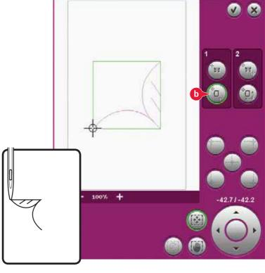
2a. To line up the design on the screen with the previously embroidered, select matching point on screen (a) to be the corner. Use the touch function - move or the corner icons.
