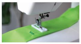
**Four-Step Buttonhole** - Sewing a perfect buttonhole is easier than ever! All four sides are stitched out in just the right size.
