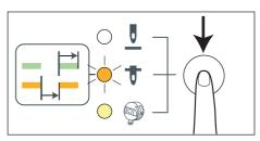
Double click the positioning button. The needle will remain in the down position and the green LED will flash on and off.
