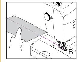
**NOTE:** When the machine is stopped and the green LED light is lit the machine will complete the cycle by taking a stitch when the positioning button is pressed to raise the needle.
