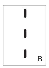
If you prefer a short stitch length and a long space between stitches then set the stitch length lever on 2 and the stitch spacing lever on 5. (Fig. B)
