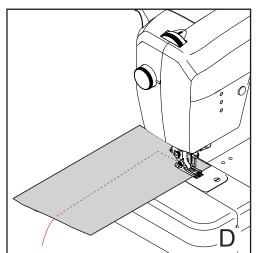
When the presser foot height adjustment dial is set at "0" to "1" the fabric cannot be pivoted without raising the presser foot.
