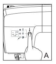
1. Press and hold the positioning button for approximately 2 seconds to set the machine to the bobbin loading position. (Fig. A)
