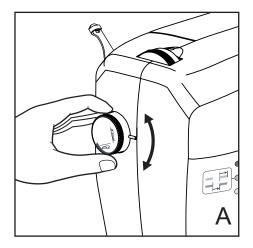
The presser foot height adjustment dial actually has two functions - straight sewing or curved sewing. This dial is located on the left side of the machine.
