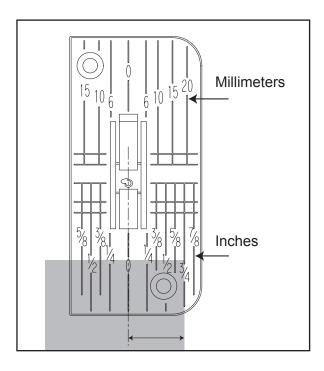
Using the needle plate scale will allow ease of maintaining an equal sewing distance from the needle to the fabric edge.
