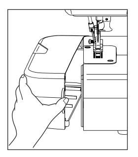
To open for threading grasp the side cover located on the left side of the machine and pull as illustrated.
