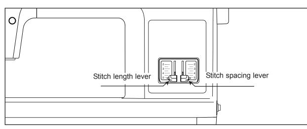
The stitch length lever and the stitch spacing lever are conveniently located on the right side of the front panel. You will notice there are two sets of numbers ranging from 2 (shortest) through 5 (longest) for each lever. One range is for the stitch length, which forms the actual stitch on top of the fabric. The other one is for the stitch spacing, which is the distance between the actual stitches.
