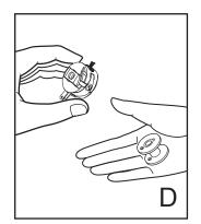
5. To remove the bobbin from the bobbin case release the hinged latch of the bobbin case. (Fig. D)
