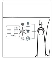
Double click the positioning button. The needle will remain in the down position and the green LED will flash on and off.
