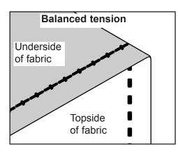
The Sashiko stitch has the correct thread tension when the actual stitch sewn on the topside of the fabric lays straight and shows no fabric puckering around the stitch.
