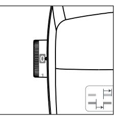
**REMINDER:** While the needle is set in the up position a space and actual stitch can be made by pressing the foot control one time. The foot control will need to be pressed twice when the needle is set in the down position.
