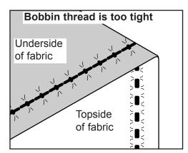
The bobbin thread is too tight when the stitches pull the fabric and create puckers on the underside or topside of the fabric.
