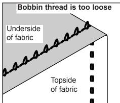
The bobbin thread is too loose when thread loops form on the underside of the fabric. On the topside of the fabric, where the actual stitch is formed, the two threads may separate.
