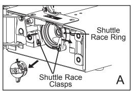
Remove the bobbin case from the shuttle race pin and push the shuttle race clasps toward the outside edges of the shuttle race ring. (Fig. A)
