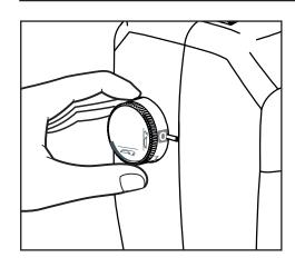
Align the presser foot height adjustment dial with the notch on the machine to "0" for the straight sewing position.
