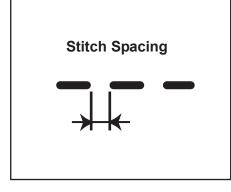
Slide the stitch spacing lever up or down to the desired setting by aligning the lever's pointed extension with the marking indicated on the machine. The spacing is adjusted only for the distance between the actual stitches sewn on the top of the fabric.
