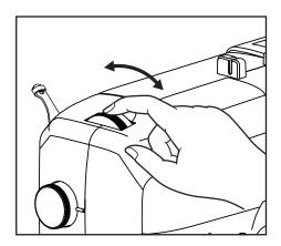
The presser foot pressure adjustment dial has been preset at the factory and rarely needs adjustment. You may find it necessary, however, to decrease the pressure for heavy fabrics or increase pressure for thin fabrics to feed more smoothly under the foot.
