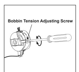
Turn the bobbin tension adjusting screw of the bobbin case counterclockwise to loosen the bobbin thread or turn the screw clockwise to tighten.
