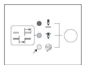
3. When machine is set to the loading position and presser foot is in the raised position.
