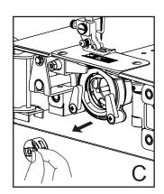
4. Remove the bobbin case with the bobbin from the machine. (Fig. C)
