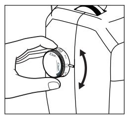
Align the presser foot height adjustment dial with the notch on the machine to one of the numbers ranging from 1 through 3 for the curved sewing position.
