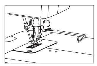
To use the quilting guide, loosen the quilt guide fixing screw located on the back of the presser foot holder. Insert the straight end of the guide into the right side of the hole opening.
