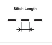
Slide the stitch length lever up or down to the desired setting by aligning the lever's pointed extension with the marking indicated on the machine. The length is adjusted only for the stitch sewn on the top of the fabric.
