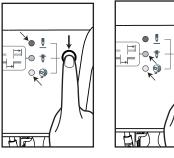
Press and hold the positioning button for approximately 2 seconds and the machine will automatically move to the loading position. The yellow LED light will now be lit.
