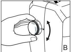
When the presser foot height adjustment dial is set at 1-1/2 to 3 the fabric can be pivoted without the need to raise the presser foot. Follow the steps below for pivoting your fabric properly when curved sewing.
