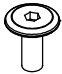
M6 x 12mm Socketed Washer Head Cap Screw, Track Support Screws (12) (Comes in track supports on table sections) QF09318-303 Box 1
