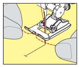
> Pull both cord ends under the buttonhole foot to the back and place each cord into one of the grooves of the sole.
