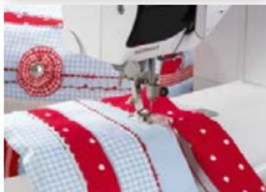
With the assistance of the Spanish hemstitch equipment edges can be joined in a defined distance and decorative edge finishings with borders can be sewn.
