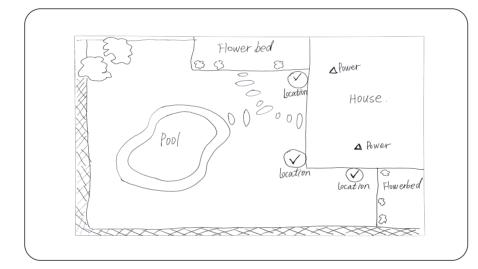
2. Sketch your lawn area. Identify and mark any objects that are to be excluded from the cutting area such as tress, flower beds, ponds, which will help with the wire layout. Mark a power socket and choose a suitable and flat location for the charging station.
