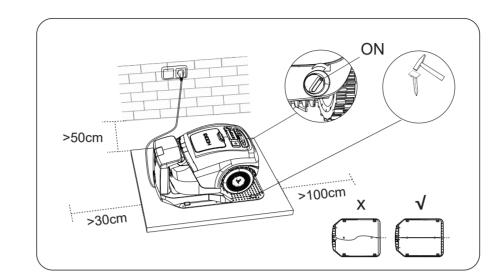
4. Install the charging station with the nails, and feed the power supply cable into the charging station. Switch the ON/OFF key to on, then place the mower on the charging station to charge.
