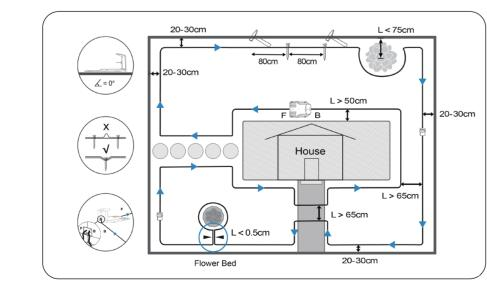
3. Install the boundary wire clockwise and connect the wire to the charging station. (Note: Please refer to the picture for more details )
