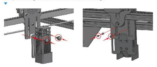
The screw passes through the isolation cylinder, after installation, the laser head can move up and down is better.
