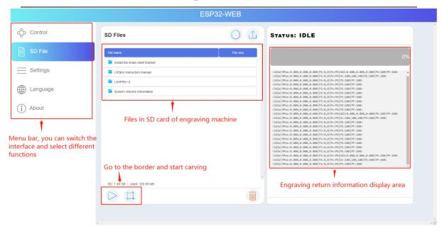
h) Upload .gcode/.nc files generated by "LaserGRBL" or "LightBurn" software(The two software are introduced in the following sections). Then go and play!
