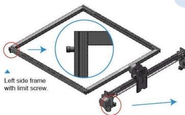
Pay attention to adjusting the eccentric nut to prevent the roller from being damaged by the groove.
