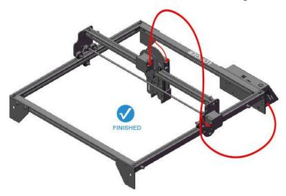
Note: Fix the cable with a cable tie and sheet metal to ensure that the cable has enough length to ensure that the length of the cable is sufficient for the laser head to move to the limit position.
